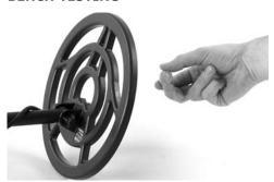
This will enable you to test typical targets and to learn about the discriminating capabilities of the GTI before taking it into the field or trying to set discrimination. The following tests should be performed, as shown above with the searchcoil perpendicular to a bench, floor or other nonmetallic surface and several feet away from any metallic object:
