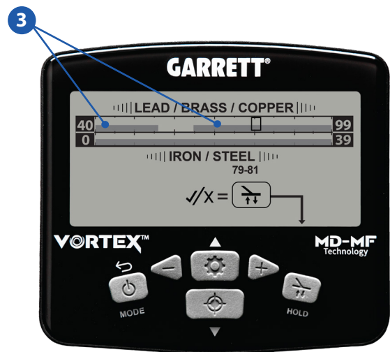
Figure 2: Tap Menu and navigate to Notch Discrimination controls if you wish to further narrow the accepted or “good” target range.
