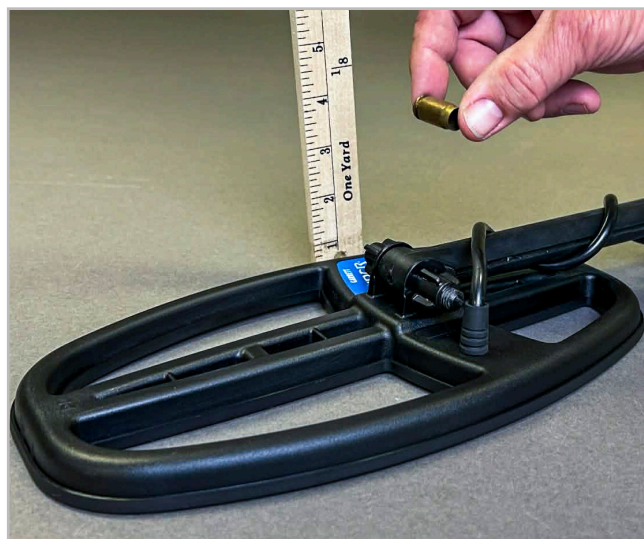
For bench testing, place the searchcoil on a flat, stable, and non-metallic surface that is several feet from other metallic objects.
