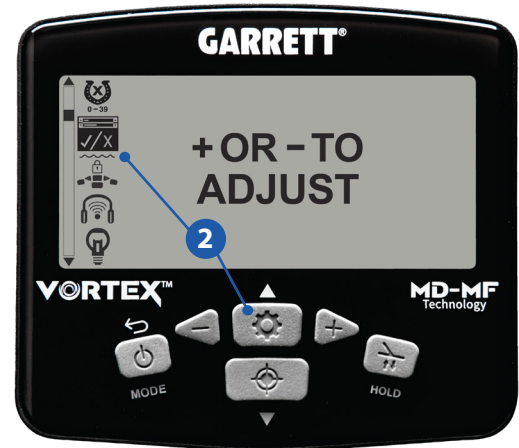
Figure 2: Tap Menu and navigate to Notch Discrimination controls if you wish to further narrow the accepted or “good” target range.
