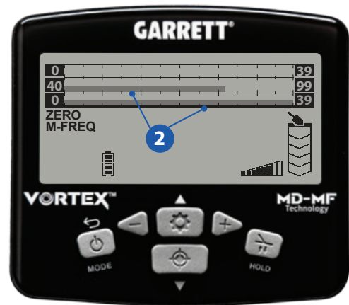
Figure 2: This LCD indicates any Target ID of 81 or less will produce a low tone (all areas partially grayed-out at half-height).
