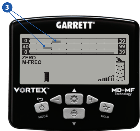
Figure 3: Use both High Res Iron Discrim and Notch Discrim to convert any undesired target areas to a low tone. This LCD indicates a high level on iron discrim on the lower ferrous Target ID scale, and other specific discrim blocks applied to the upper two Target ID scales.
