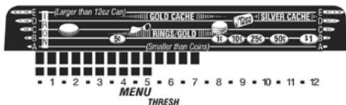
Pressing the MENU touchpad to display THRESH on the screen (below, with factory setting indicated on Upper and Lower Scales). Use the (+) and (-) touchpads to adjust the threshold of sound that is being produced by the *GTI 2500* as it scans. Multiple touches will increase or decrease the sound level. Changes can be seen on the Upper and Lower Scales.
