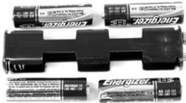
7. Replace holders in detector as shown above. It is important that the "eyelets" be toward the center. If an effort is made to install holders incorrectly, closure will be difficult. If it is forced, however, damage to the detector can result. Battery packs must be replaced in their proper orientation.
