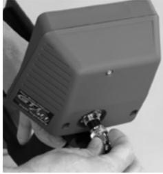
slightly loose (*above left*) so that the angle of the searchcoil can be changed easily, if required. Insert the cable connector into the connector on the control housing as shown (*above right*) and rotate the collar clockwise until secure (approximately four (4) turns). Hand tighten only.
