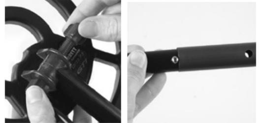
2. Place the threaded bolt through the holes in the connector and hand-tighten using the remaining wing nut (*above left*). Use no tools.
