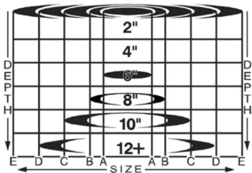
A at 6"; a Size B at 8"; a Size C at 10"; or a Size D at 12". The Cone may also appear when the target is significantly off-center from the coil.
