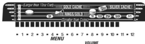
After pressing the MENU touchpad to display **VOLUME** on the screen, the factory setting for the loudness of the target sound will be indicated on the Upper Scale, as shown in the above diagram.
