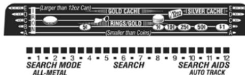
After you press this touchpad, the Graphic Display will indicate that you are operating in an all metal (deepseeking) mode. Garrett's exclusive *Fast Track* feature can be used to ground balance your detector automatically, and *Auto Track* can continually work to keep it ground balanced over varying soil mineralization conditions.
