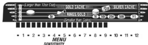
Pressing the MENU touchpad to display SENSITIVITY on the screen (shown above with factory setting at approximately 75% as indicated on the Upper Scale). Use the (+) and (-) touchpads to adjust the depth to which your detector will operate most effectively. These changes will be shown on the Upper Scale as you make them.
