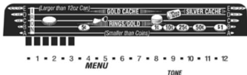
After using the MENU touchpad to display TONE on the screen, the factory tone setting will be indicated on the Upper Scale, as shown above. Use the (+) and (-) touchpads to adjust the audio to preferred pitch or tone. Touching the (+) pad will raise the tone into a higher treble range, while touching (-) will lower the pitch to a bass tone. All touches will make changes indicated on the Upper Scale. Experiment to find the pitch that suits your hearing.
