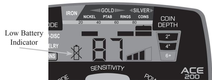
The Low Battery Indicator will switch on when the detector's batteries become weak. The detector will maintain full performance but the batteries should be replaced soon when this indicator appears. NiMH rechargeable batteries may be used, but may have a shorter life per charge. You can expect 20 to 40 hours of operation depending on battery type and quality.
