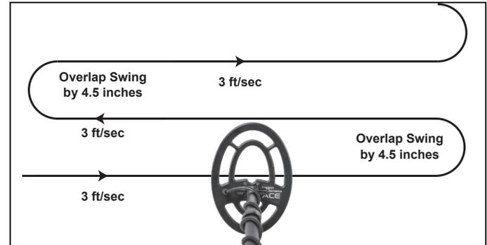
In order to fully search an area, overlap the swings of your searchcoil by half the length of the coil (about 4.5 inches). Sweep the searchcoil in a straight line or with a slight arc at a sweep speed of about 3 ft/sec.
