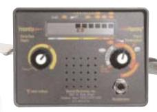
Clear signals on the Ace 300 LCD provide instant Visual Target ID. Its LCD panel has twin scales. The upper scale indicates the full-range discrimination
