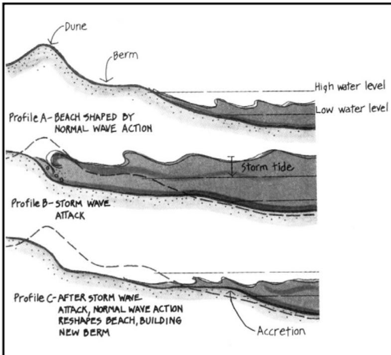
Storm tides can completely reshape sand dunes on beaches, as shown in this illustration from a booklet produced by the U.S. Army Corps of Engineers.
