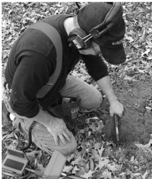
A quality hand-held pinpoint detector can save considerable time in determining if your coin is still in the ground or in the dirt pile that you have removed.
