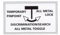
**A.** When the ALL METAL toggle is in the temporary or LOCK position the instrument responds to all types of common metals. Note that some loop movement is required.
