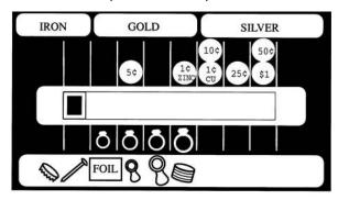
This block indicates the metal is likely iron or steel such as nails, steel bottle caps, or iron relics. Dig only if iron/steel is of interest.
