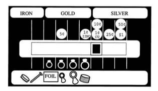
The most common metals found with this block indication is medium to large copper and silver coins. Other items of copper/silver can also be indicated by this block. We recommend digging this indication.
