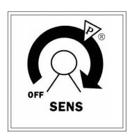
clockwise, detection depth as well as sensitivity to physically small metal items increases. Unfortunately, external electrical interference and ground interference also increases. The best setting is the furthest clockwise position that provides smooth, stable and predictable results.
