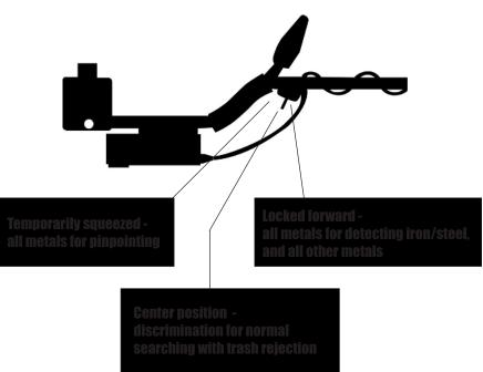
**IX.** If the desire is to detect iron/steel such as tools, relics or property stakes, place the ALL METAL toggle in the forward LOCK position and leave it there during searching. With the ALL METAL toggle in the forward LOCK position, all types of common metals respond.
