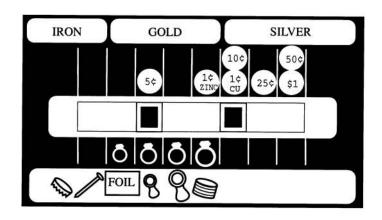
VII. Once a smooth consistent beep has been located, sweep the loop directly over the center of the target several times and read the possible ID on the display. Like the audio discriminator, the display will tend to fluctuate on trash, and read more consistent on valuable metals. This is why we recommend relying on the audio beep as the primary indication, and then check the display ID.
