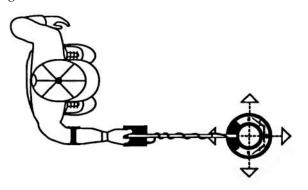
**A.** Note that some loop movement is required. It is a good idea to place coins on the ground and practice pinpointing. It takes some time to develop pinpointing skills. Release the ALL METAL toggle and it will automatically return to the DISC position before continuing to search.
