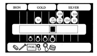
The most common metals found with this block indication may either be medium copper or zinc coins or the large aluminum screw off bottle cap depending on the area. However, larger gold jewelry can also be indicated by this block. In areas where rings are suspected, you may want to dig these indications, at least until you have determined the presence of many screw caps.
