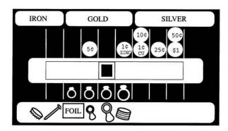
The most common metal found with this block indication is the standard size "PULL TAB". However, medium to larger gold jewelry can also be indicated by this block. Again in areas where rings are suspected you may want to dig this indication, at least until you have determined the presence of many pull tabs. The DISC control at high settings can reject metals with the audio sound that produce this display indication.
