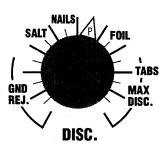
VI. DISC: The Discrimination control selects the amount of rejection against junk metals such as nails, tin or aluminum foil, etc. It only affects the GEB/DISC and TR/DISC MODES.
