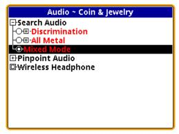
Without mixed-mode, you can hear either the all-metal audio or the discrimination audio. The all-metal channel doesn't tell you anything about the quality of a target; the discrimination channel only signals on accepted targets, and rejected targets cause a null in the audio. Weak targets below the discrimination threshold produce no discrimination response.
