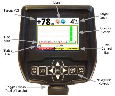
signal strength versus VDI and gives a detailed look at the VDI response. The status bar shows a few operational pieces of information, and the Live Control Bar provides quick on-the-fly access to operating modes and adjustment parameters. All of these will be covered in detail in subsequent chapters.
