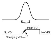
In three frequency mode the VDI is a composite number based on the peak VDI readings of at least the two strongest responding frequencies. For that reason, you may occasionally notice that the VDI number does not exactly match the Spectra-Graph response, especially for a weak frequency. In single frequency mode the VDI is obviously taken off the one active frequency.
