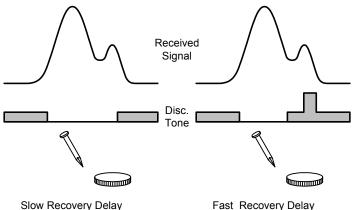
The recovery delay determines how long the disc response (tone or null) lasts. A longer delay results in a longer response. In trashy sites, a long response delay can mask targets that are close to rejected trash. Even good targets close to each other will be difficult to separate. A short response (shorter recovery delay) makes it easier to separate close targets.
