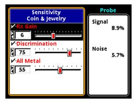
On the right side of the screen are two live "signal quality" numbers. The "Signal" number tells you what percent of the total signal range is currently being received; that is, how much
