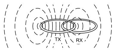
reaction. A so-called "induction-balanced" coil arrangement prevents the receive coil from being overwhelmed by the transmit signal, allowing it to see very small target signals.
