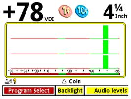
1. Programs which run in single frequency mode will display a single frequency SpectraGraph.
