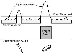
When mixed-mode is selected, there are no additional settings. By default, Tone ID is on, modulation is set to 1, and allmetal VCO is on.
