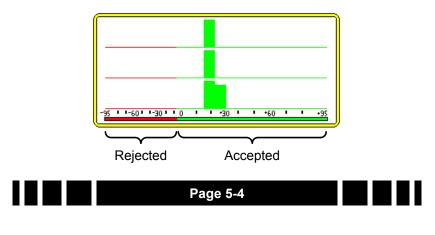
Ideally all targets would have tight responses that are repeatable. The closest you can get to that is to air test targets 3-4" from the coil, and that is not a bad start to learn how different targets respond. However, just like we discussed with VDI numbers, as a given target moves farther from the coil, its response gets weaker and exhibits shifts and spreading in the graph response, and is not as repeatable. This gets even worse in mineralized ground.
