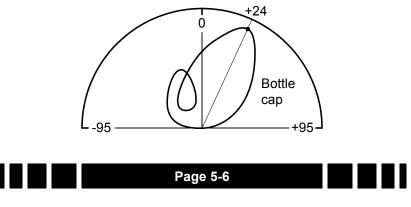
As the loop is swept over the bottle cap, the phase response varies wildly. This will not only result in smearing of the Spectra-Graph plot, but will also cause it to jump around significantly before it locks on to a final reading. Such a final reading might look like:
