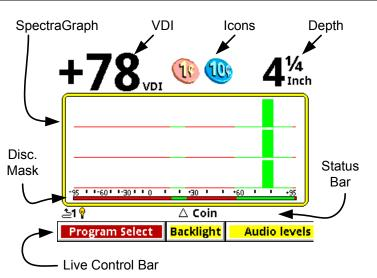
The Search screen has several regions as labeled above. The central part of the screen is the SpectraGraph which plots the target response in terms of signal strength versus VDI. In the screen shown, there are three of these responses, one for each frequency. The top region shows the (composite) VDI readout, icons, and depth. The "status bar" shows a few status icons and other information. The Live Control Bar has been covered in previous chapters.
