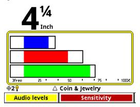
Again, this screen has the depth (but no VDI or icons), Status Line, and Live Control Bar. The Pinpoint display consists of 3 horizontal moving bars<sup>2</sup> which give the relative signal strengths of the three frequencies. This can be used to precisely pinpoint the target, and to see which frequency is giving the strongest
