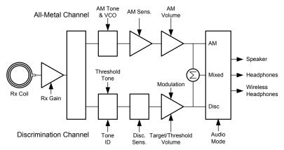
the raw input signal from the coil. The signal is then split into two processing channels, one for all-metal and one for discrimination, and these channels have their own audio responses.  $VX^3$  has the following three search audio modes:
