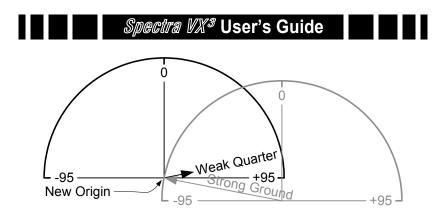
Any error in the ground balance point can result in an error in the target VDI response so it's important to maintain a decent ground balance point.
