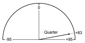
This might represent a somewhat shallow quarter, and would have a SpectraGraph response with nice tight bars. Note the black dot, which indicates the peak signal strength; this is also the point where the VDI number is calculated. The same quarter buried deeper begins to exhibit a small amount of curvature in the vector response:
