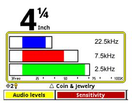
The Pinpoint screen has regions similar to the Search screen, and is accessed by pulling the trigger switch. The central part of the screen is the Pinpoint bars which show the live signal strength of the received signal, regardless of what causes it. In the screen shown, there are three of these responses, one for each frequency, again with the highest frequency on top. The top region shows depth. The same status bar and Live Control Bar are also displayed.
