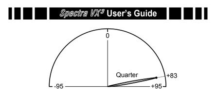
Now the signal response starts at zero and still reaches approximately the same peak point (perhaps resulting in the same final VDI), but shows some curvature on the way up and on the way back. Because the SpectraGraph response is taken from the whole of the signal response and not just the peak, this can result in a "smearing" effect in the bars, as shown here:
