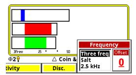
While continuing to hold the trigger, select **Transmit Frequency** and highlight the **Offset** box. Adjust the **Offset** to find the quietest setting. The pinpoint bars should be minimal and steady:
