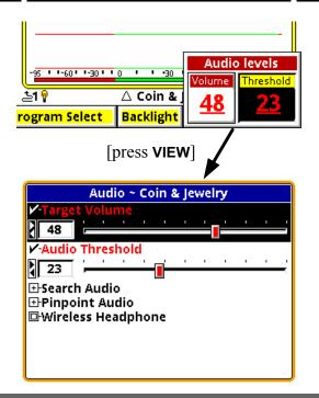
Tip: The Live Control Bar is the collection of buttons across the bottom of the screen. Each button is called a Live Control Item. Each item consists of one or more settings. Press VIEW for any Live Control Item to access a Menu for that item. Keep in mind that the detector is "live" while accessing the Live Control Bar, but is suspended when you enter a Menu.
