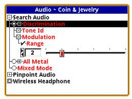
**Tip:** Modulation is most effective when you want to distinguish between deep and shallow targets of similar type. For example, if shallow coins are likely to be clad and deep coins are likely to be silver, then modulation will give you that information in the audio response.
