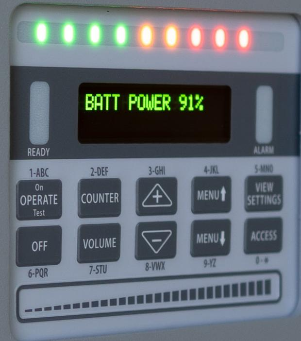
Each Garrett Multi Zone walkthrough includes a 1-hour emergency backup battery module. Keep your checkpoint functional in the event of a power outage or AC power disconnect. (A 10-hour operation battery is also available.)
